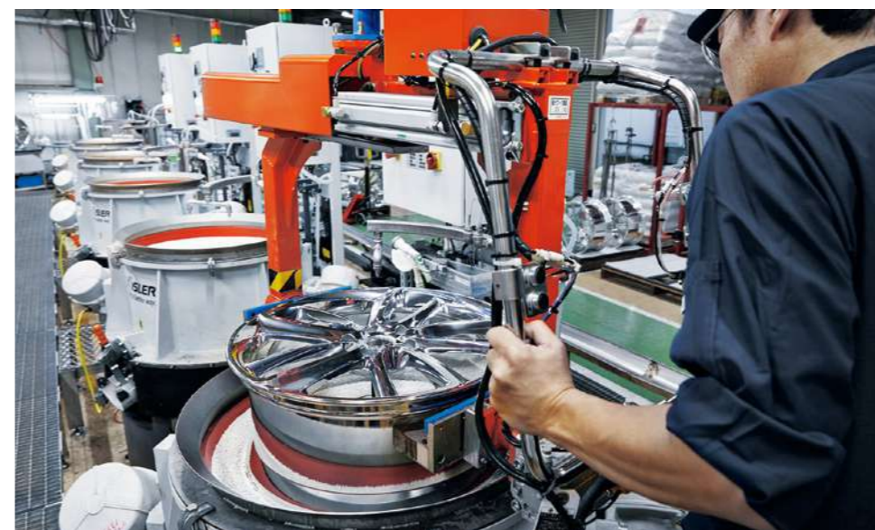
Making wheels shine while ensuring their strength. A craftsman checks the finish of a wheel.
